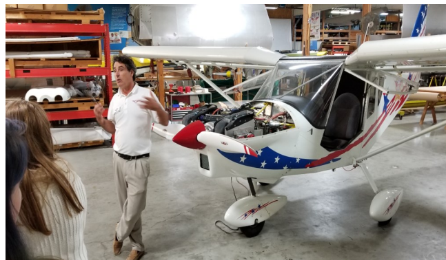
Zenith airplane is shipped in wooden crate and assembled by the buyer.
